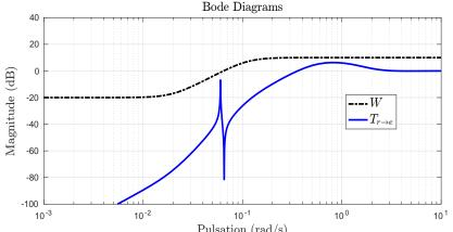
Frequency constraint on  $e(i\omega)$ : we want  $|\frac{e(i\omega)}{r(i\omega)}| = |T_{r\to e}(K, i\omega)|$ to be small
