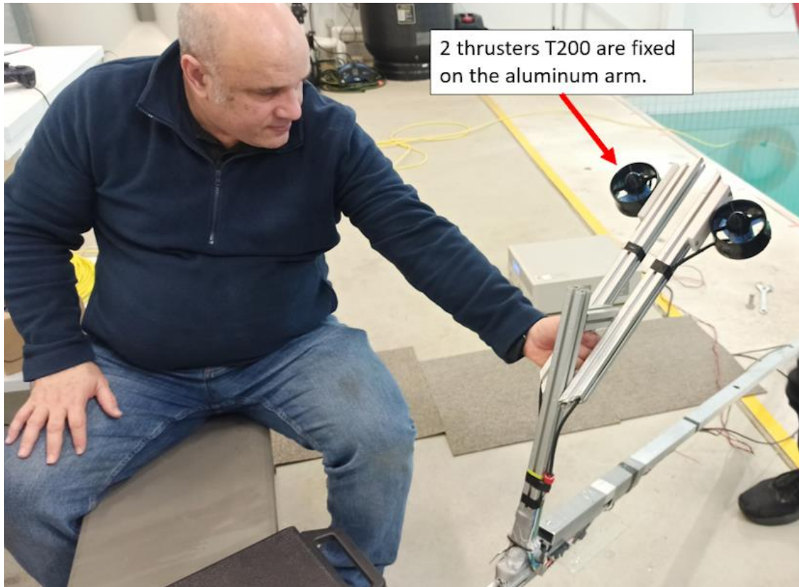
Illustration of the disturbance generator and tracking system for pose estimation.
