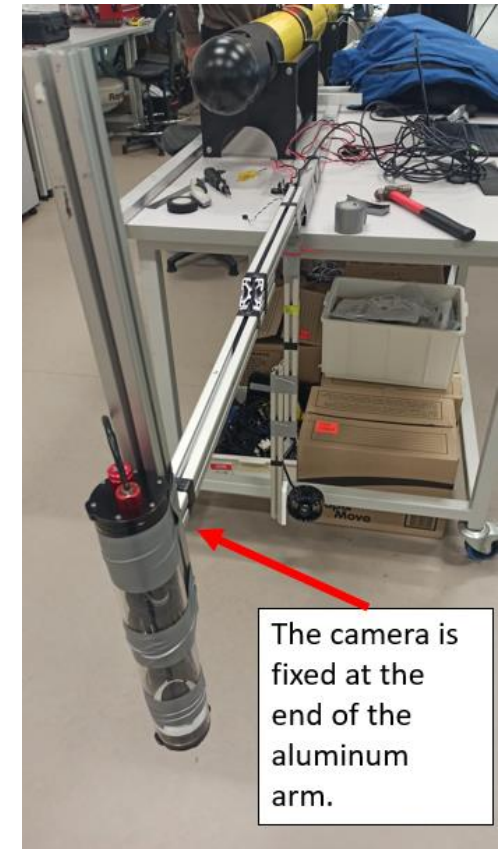
Illustration of the disturbance generator and tracking system for pose estimation.
